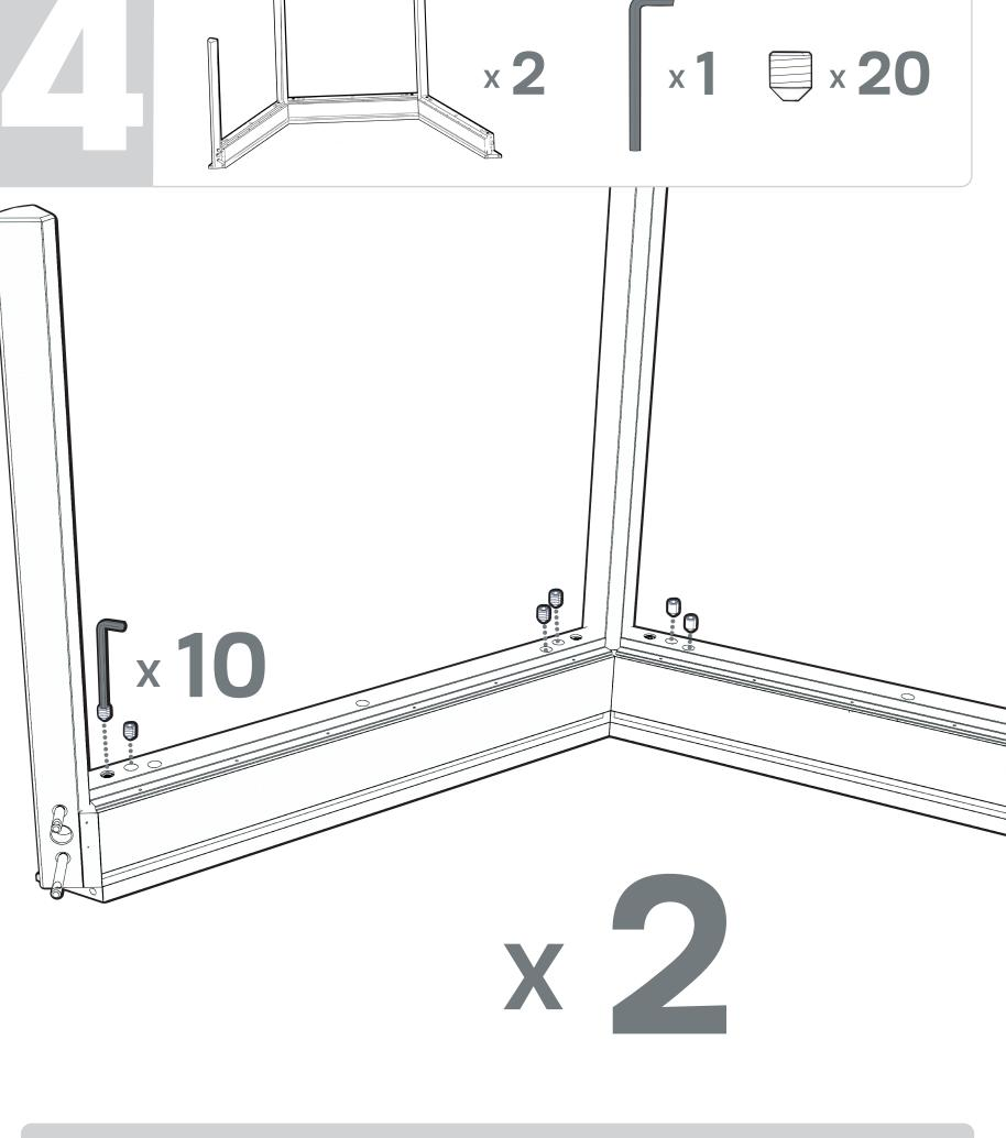
Don't overtighten Grub Screws. Keep joints loose to ensure a snug fit during the next step.
