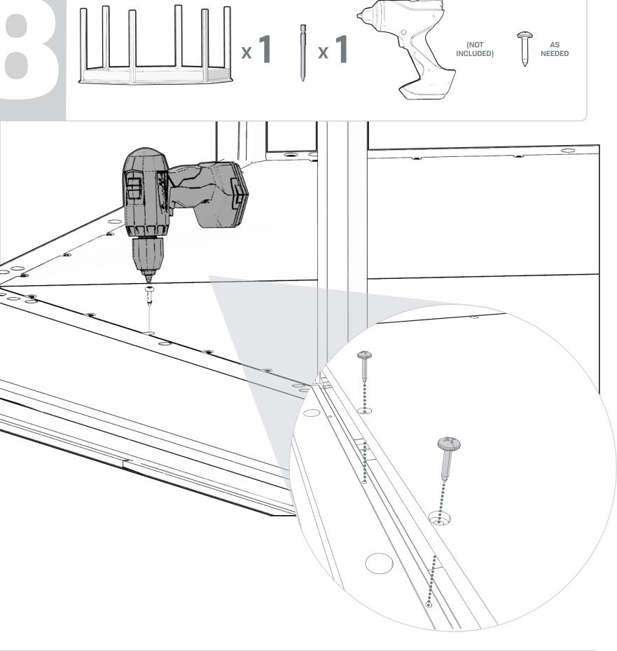
To avoid damaging the plywood, avoid overdrilling wood screws. Use pilot holes as a guide when drilling, but it's okay if they're not perfectly aligned.
