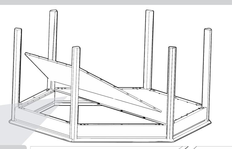
Tighten all the Grub Screws after fitting the two halves together.
