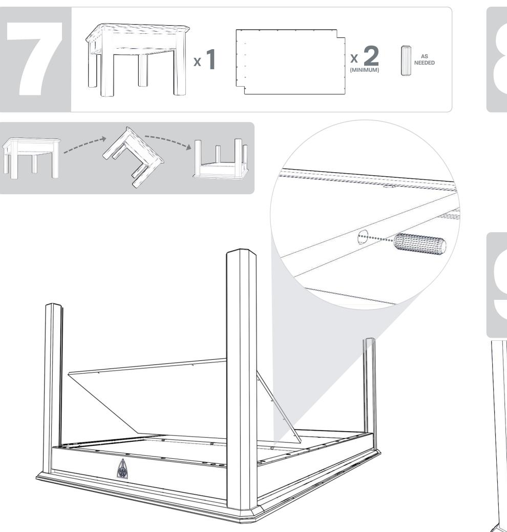
Ensure each Plywood Panel is placed into the Table Frame • with countersinks facing up
