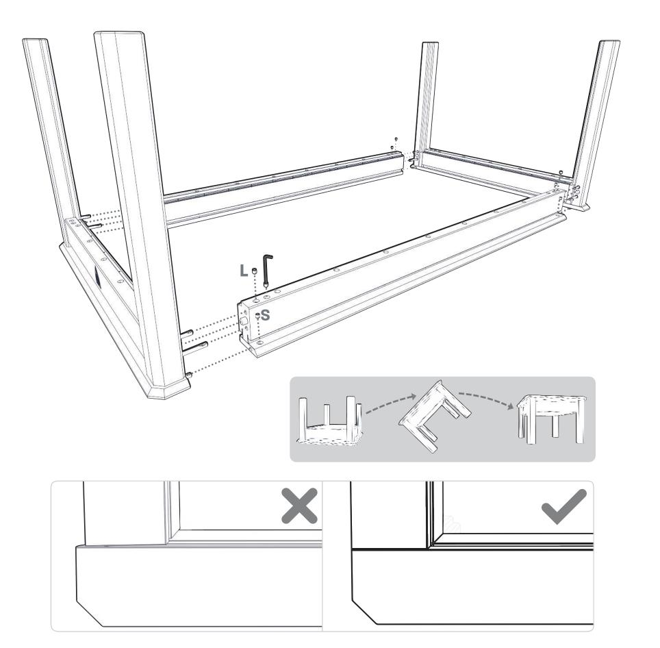
Check apron alignment before moving on to the next step
